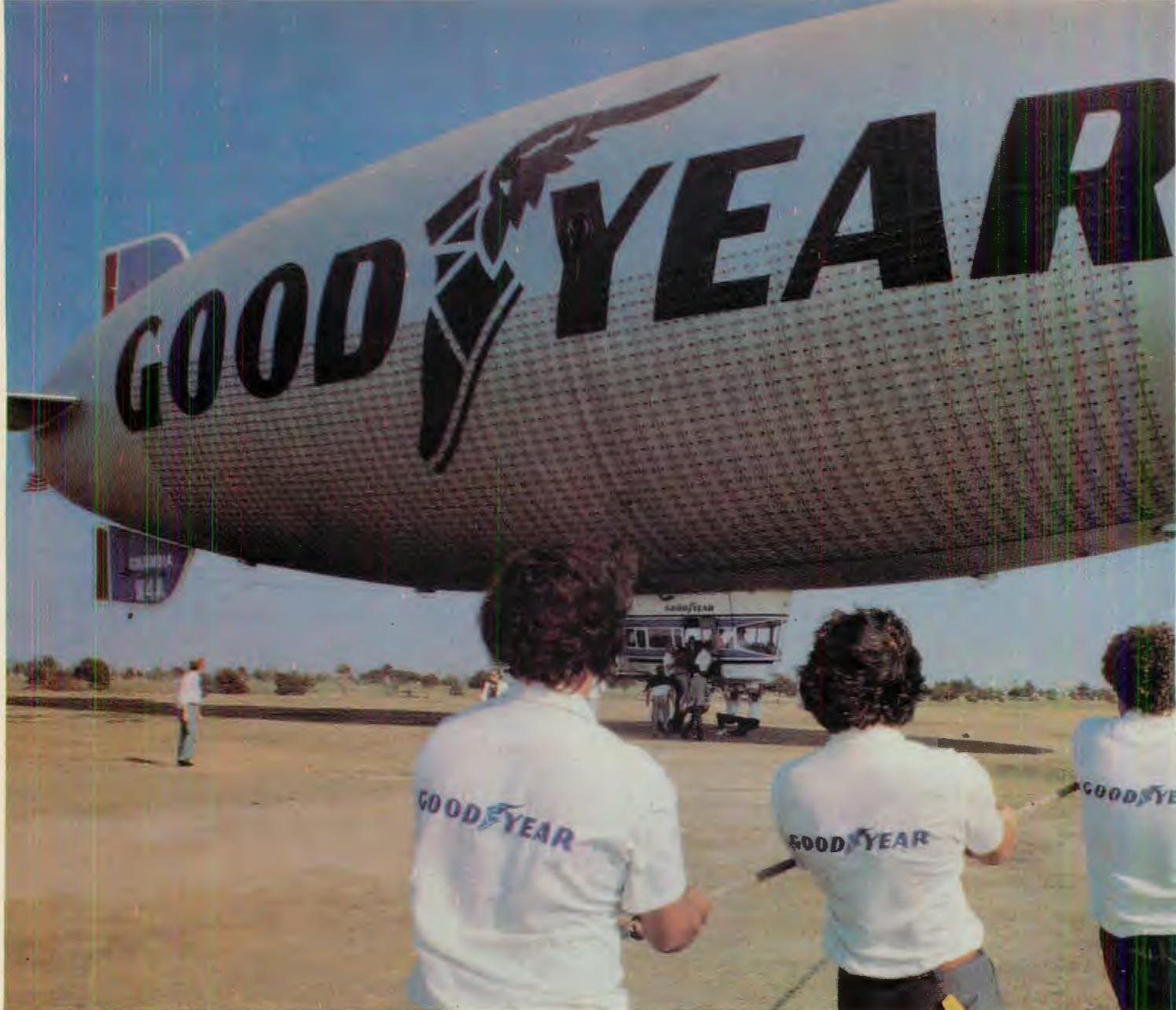
ABOVE: Crew readies airship for launching by holding lightweight ship down as pilot brings nose into wind. RIGHT: After launch, crew breaks down mooring mast, before storing it underground.
